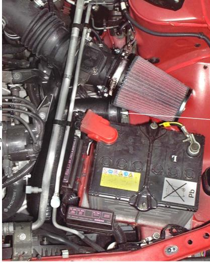
2. Position the end of the flexi cold air hose to finish 10cm / 4" from the filter no nearer.
