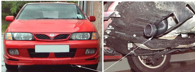
Feed the flexi cold air hose down and through the gap in the undertray. Drill two 3mm holes in the undertray and secure the end of the flexi cold air hose to it using a long plastic tie supplied.
