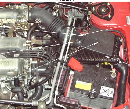
**4.** Remove the MAS from the air box lid by removing the 4 bolts.
