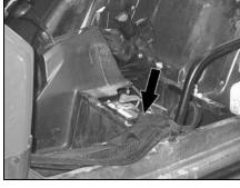
3. Disconnect the vehicle's negative battery cable.
