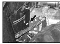
20. Install the lower air box bracket (#09496) onto the shifter cable bracket at the left side of the transmission as shown.
