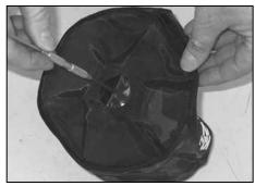
29. Using a sharp tool, poke a hole in the center of the reinforcement patch on the K&N® Drycharger®.
