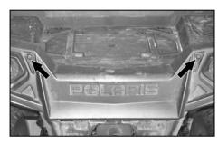
8. Remove the two torx bolts at the rear of the cargo bed as shown.
