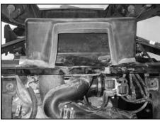
33. Re-install the plastic intake cover using the factory clips (removed in step #12).
