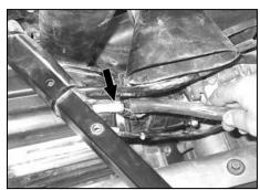
16. Remove the crank case vent hose from the air box assembly as shown.
