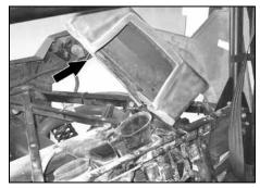
14. Remove the intake cover as shown.
