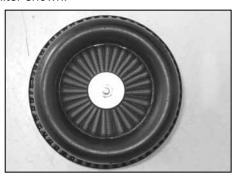
28. Install the provided bolt through the air filter top and secure it with the provided hardware as shown.
