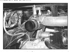
21. Install the K&N® intake tube into the factory rubber manifold and secure with the factory clamp removed in step #18 as shown.
