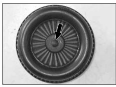
27. Remove the rubber plug from the top of the air filter shown.
