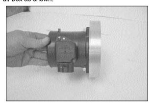
26. Assemble the filter adaptor and gaskets onto the mass air sensor with the provided hardware as shown.
