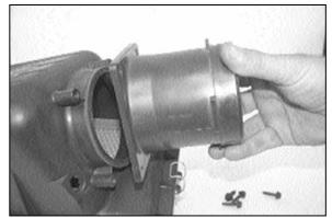
25. Remove the mass air sensor from the factory air box as shown.
