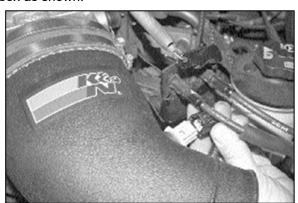
24. Install the temp sensor into the intake tube then reconnect the electrical connection as shown.
