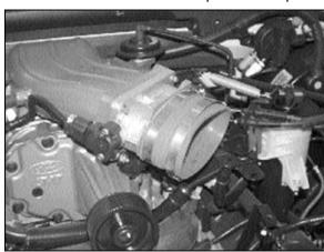
15. Install the silicone hose (08540) onto the throttle body with the provided hose clamp as shown.
