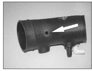
17. Install the provided grommet into the new intake tube as shown.
