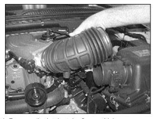
4. Remove the intake tube from vehicle.
