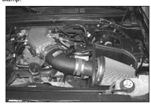
31. It may be necessary to loosen the hardware and adjust the entire assembly to achieve proper clearances.
