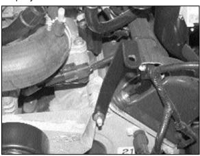
14. Install the provided bracket onto the stud with the nut that was removed in the previous step.
