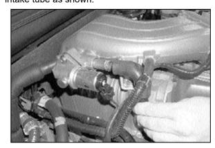
18. Remove the idle air vent tube from vehicle as shown.
