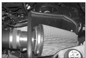
30. Install the Filtercharger onto the mass air adaptor and then secure it with the provided hose clamp.
