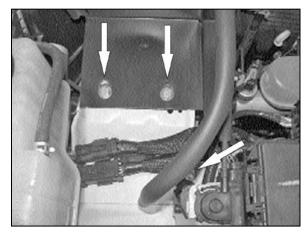
12. Install the heat shield into vehicle, then secure with the provided hardware as shown.
