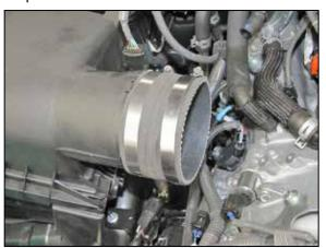
8. Install the provided coupling hose (08760) onto the air box lid as shown and secure with the provided hose clamps.
