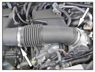
4. Loosen the two hose clamps securing the factory intake tube to the throttle body and air filter housing and then remove the factory intake tube.
