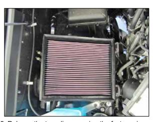
5. Release the two clips securing the factory air box lid and then remove the factory air filter. Install the provided K&N® air filter into the air box, set the air box lid into position but do not secure at this time.
