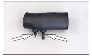
6. Install the two provided vent fittings into the  $K\&N^{\otimes}$  intake tube as shown.
