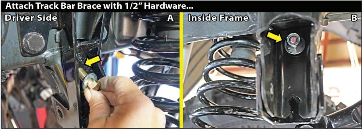
6) ATTACH TRACK BAR TO TRACK BAR BRACE & FACTORY MOUNT.. Locate Hardware Bag #77-5805. Hardware PER Side: (1) 9/16" x 3-1/2" Bolt, Coarse Thread, Grade 8, (2) 9/16" SAE Washers, & (1) 9/16" Nyloc Nut, Coarse Thread, Grade 5
