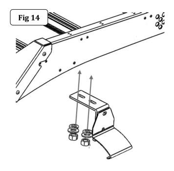
**Step-11** Adjust and align the Ceros roof rack assembly as necessary and fully tighten all hardware.
