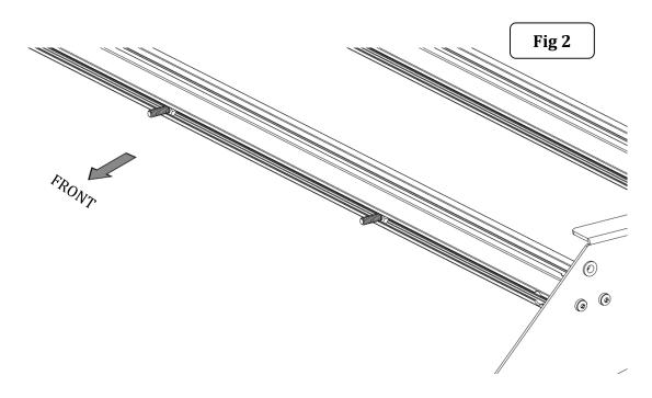
**Step-4** Position the front cover in place, align the holes in the front cover with the rivet-nuts in the side rails and align the  $\frac{1}{4}$ " hex bolt installed in the crossbar with the hole in the front cover bracket . Attach each side of the front cover to the side rail using (2)  $\frac{1}{4}$ " x 1" Allen Sems bolt. Attach to the front cover to the front crossbar using (3)  $\frac{1}{4}$ " hex nut and  $\frac{1}{4}$ " lock washer, (Fig 3 & 4). Tighten the screws and nut.
