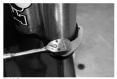
Fig. 8: Spanner wrench tighten
