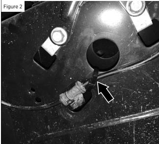
Secure the passenger side loose coil wire by attaching it to the available electrical wire routing in the upper right portion of the wheel well.
