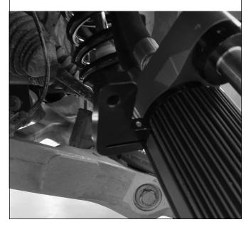
Hold the reservoir in place and use the provided 3/16 allen socket to mount the first reservoir bracket to the body mount using the provided bracket bolt. Torque to 20 ft-lbs. (27 Nm)
