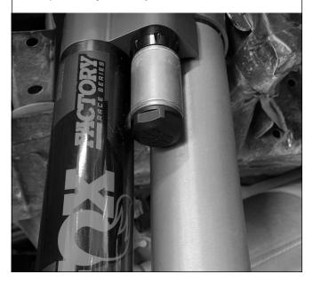
Index the Live Valve cover between the shock body and piggyback reservoir. Use a 1/8 Allen key to install one of the supplied cover bolts to secure it to the reservoir assembly. Tighten firmly.
