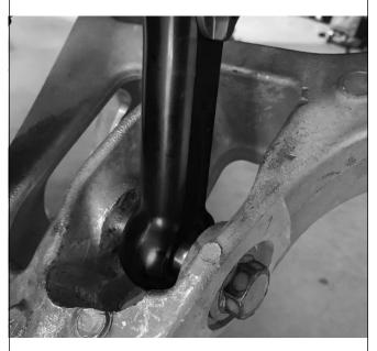
Note: The user can clock the eyelet with the switch facing away or towards the front of the truck. Rotate the eyelet to have the switch face the back of the truck if desired.
