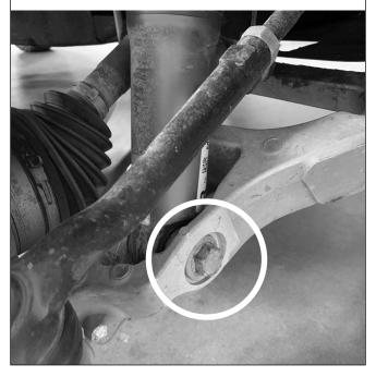
Disconnect the outer tie rod end at the knuckle using a 21 mm socket. This will provide removal/installation clearance.
