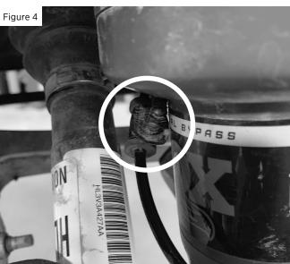
Using a 1-3/8 in. open-end wrench remove the Live Valve coil cap from the backside of the coil by turning it counter clockwise.
