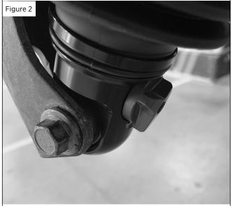
Note: The user can clock the eyelet away or toward the bracket. Rotate the eyelet and reset the boot to have the switch face the inside of the bracket if desired.
