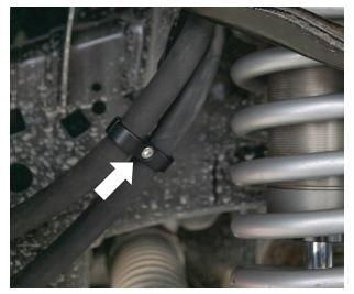
Fig. 14: Hose separator clamps.
