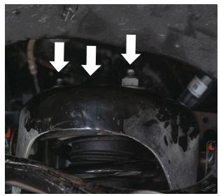
Fig. 5: Remove the three top hat nuts.
