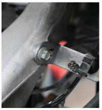
Fig. 18: Brake line bracket.
