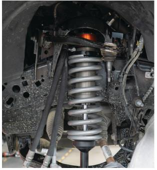
Fig. 10: The hose fitting faces inboard.
