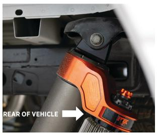
Fig. 21: Install the upper shock mount.
