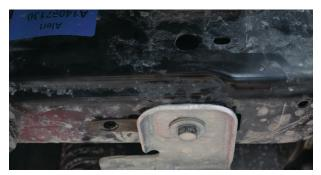
Fig. 8: Use a speed nut in front of the bracket.
