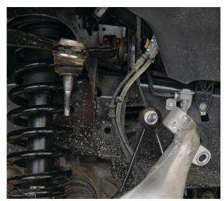
Fig. 4: Separate the UCA and upright.
