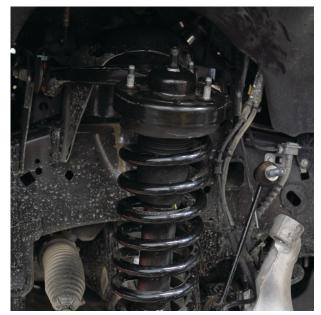
Fig. 6: Free the coil-over.
