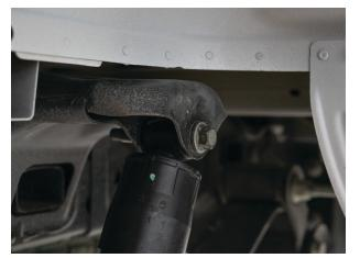
Fig. 19: Remove upper shock mount bolt.
