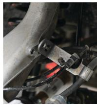
Fig. 1: Brake line bracket.
