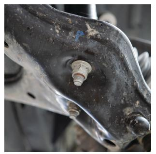
Fig. 7: Remove the bar-pin bolts.
