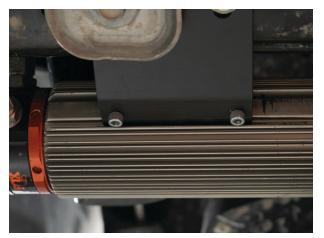
Fig. 13: Fasten the reservoir.
