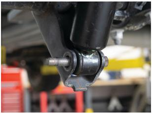
Fig. 20: Remove lower shock mount bolt.
