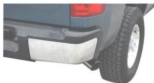
GIBSON EXHAUST systems are designed on a factory stock vehicle. Any aftermarket products installed could increase the sound levels of the exhaust. **Make sure there is a 1" clearance from ALL rubber brake lines, shock boots, lines, tires, etc. to prevent heat related damage or fire.**
