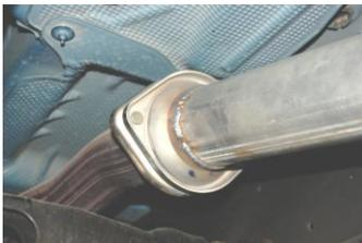
2. To remove the stock exhaust, remove it from the flange located in front of your stock muffler. Disengage the welded hangers using WD-40 from the OEM rubber grommets. Do not damage or remove the rubber grommets as you will reuse them to mount your new system. Now, cut off tailpipe and remove exhaust
