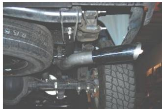
5. Install overaxle tailpipe #C into the muffler 1 1/2"-2". Insert welded hangers into rubber grommets. Use clamp #E to secure tailpipe to muffler. Do not tighten.
