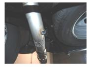
5. Adjust to fit properly then tighten all clamps and bolts. Use stainless steel cleaner to prevent tip from discoloration, Inspect all fasteners after 25-50 miles & retighten as necessary
