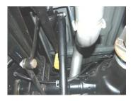
5. Install the over axle tailpipe #B onto headpipe 1.5"-2". Use clamp #D to secure. Do not Tiahten
