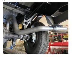
**5.** Now you may install the Over Axle Pipe #B into the muffler using Clamp #C. Then install the Tip onto the over axle to your desired location and tighten all clamps working front to back.
