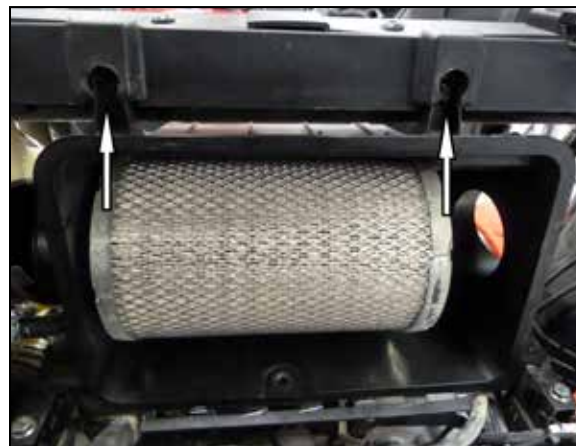
11. Remove the two bolts that secure the air filter housing to the chassis and then remove the housing from the vehicle. These bolts will be reused in a later step.
