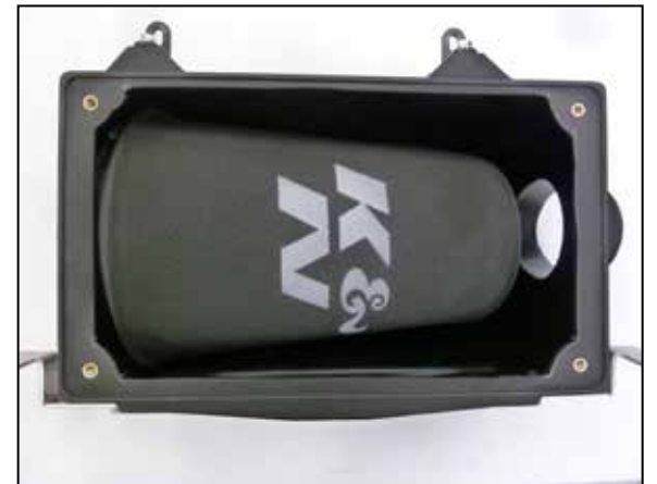
17. Install the prefilter onto the K&N air filter and then install the filter assembly onto the adapter and secure with the provided hose clamp.
