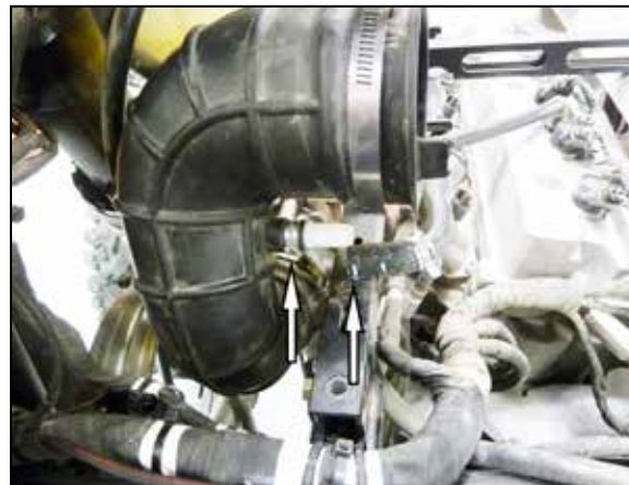
13. Disconnect the CCV hose from the factory intake tube. Loosen the clamp that secures the intake tube to the throttle body and then remove the tube.
