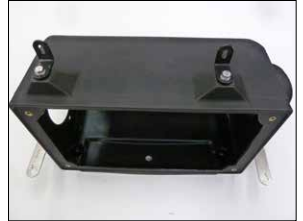
15. Install the two upper mounting brackets onto the K&N air filter housing using the provided hardware.
