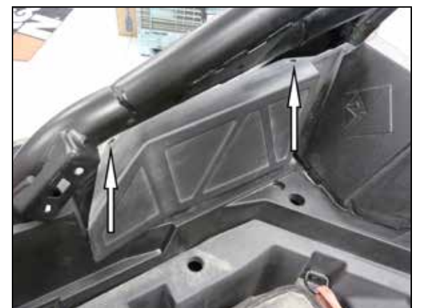
3. Remove the two pushpins that secure the left-side intake vent cover and then remove the cover.
