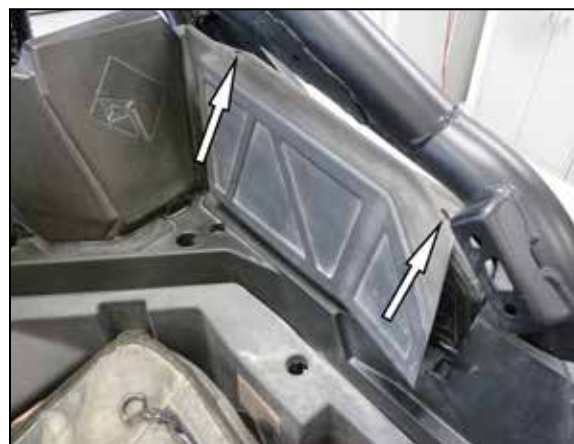
2. Remove the two pushpins that secure the right-side intake vent cover and then remove the cover.
