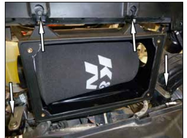
18. Install the filter housing assembly from the passenger compartment side and secure upper and lower mounting brackets with the factory hardware removed in earlier steps.
