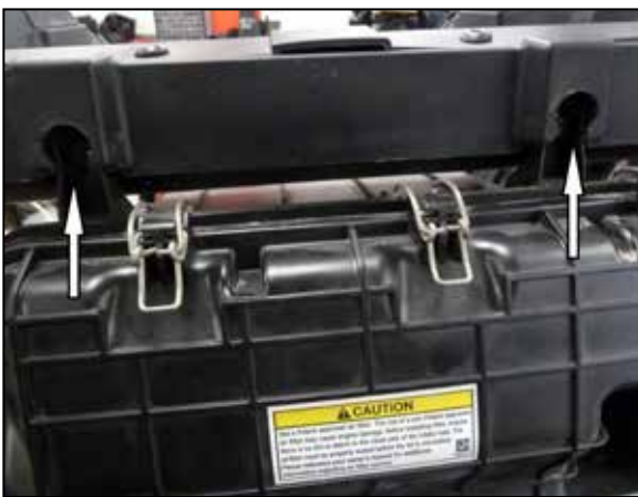
7. Using a 3/4" hole saw or similar device, drill into the trim panel to gain access to the air filter housing mounting bolts. NOTE: the bolts are just under the lip of the trim panel and easy to locate.
