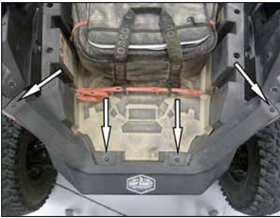
4. Remove the four bolts that secure the cargo box and then remove the cargo box.
