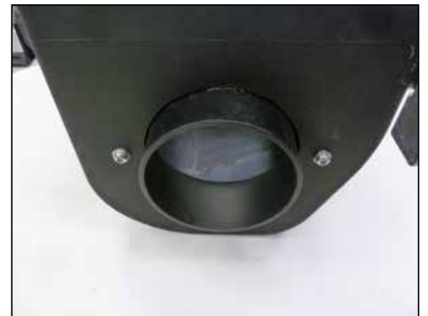
16. Install the radius filter adapter into the K&N filter housing using the provided hardware.
