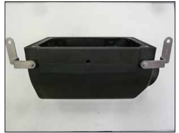
14. Install the lower mounting brackets onto the K&N air filter housing using the provided hardware.
