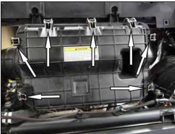
8. Release the seven over-center clamps that secure the air filter housing lid and then remove the lid.
