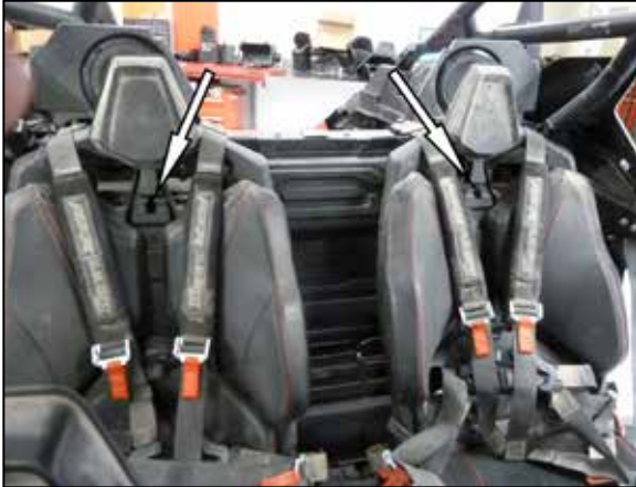
5. On four seat models, Release the latches that secure the rear seat backs and then remove the seat backs. On two seat models run the seats all the way forward.
