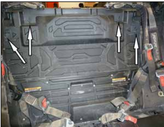
6. Release the four latches that secure the service panel and then remove the panel.
