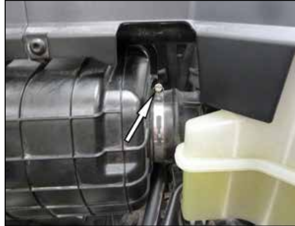
10. Loosen the clamp that secures the intake tube to the air filter housing and then remove the intake tube from the housing.
