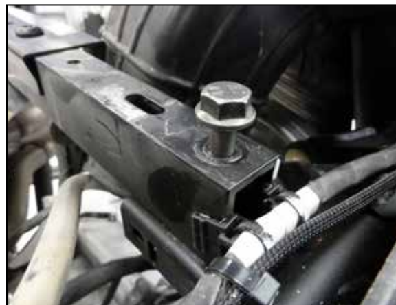
12. Remove the two large frame bolts that sit just to the left and right of the factory air filter housing. These bolts will be reused in a later step.
