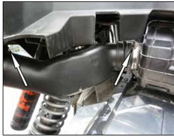
9. Loosen the clamps that secure the fresh air intake duct and then remove the duct.
