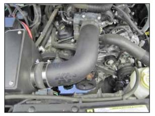
34. Install the K&N<sup>®</sup> intake tube into the hump coupler and then into the throttle body coupler, adjust the tube for best fit and then secure with the provided hose clamps. Reconnect the inlet air temperature sensor electrical connection. 39. Install the provided coupler (08284) onto the elbow secured to the air filter housing and secure with the provided hose clamp.
