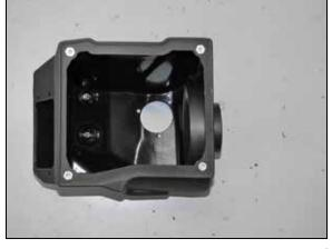
21. Using the provided hardware, secure the K&N<sup>®</sup> filter adapter to the air filter housing.
