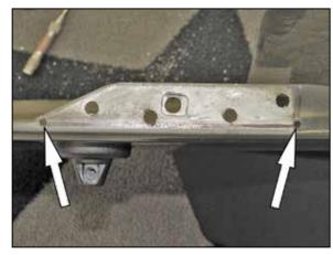
47. Drill a 3/16"id hole into each corner of the cut area as shown.
