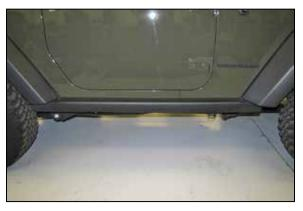
6. On vehicles equipped with rock sliders or running boards, remove the passenger side to gain access to the lower fender mounting bolts. **NOTE: The factory rock sliders secure to the body with bolts and nuts on studs.**
