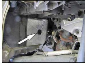
36. Remove the Insulation retaining nut shown.
