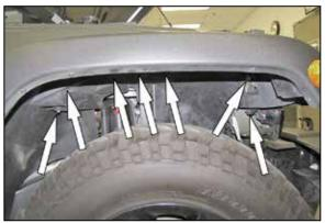
15. Remove the seven inner fender bolts.
