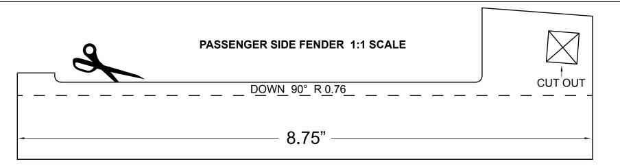
Carefully cut along outer edge of template and also cut out the square alignment hole.
