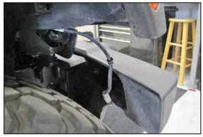
14. Remove the marker light bulb from the housing and disconnect the harness retaining clip from the fender.
