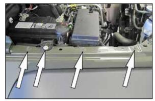
5. Lift up the air filter housing to dislodge it from the mounting grommets and then remove it from the vehicle.
