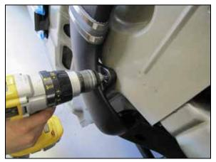
51. Adjust the corner tube and secure the hose clamps. Using the mounting hole in the corner tube as a guide, drill a 5/64" id hole into the inner body panel.
