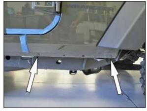
13. Remove the two lower fender bolts.
