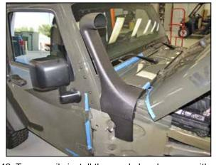
42. Temporarily install the snorkel and secure with the factory cowl bolts. **NOTE: The snorkel will be removed in a later**
