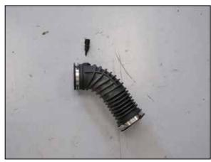
32. Remove the inlet air temperature sensor from the factory intake tube.
