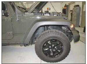
55. Reinstall the fender and secure with the factory
