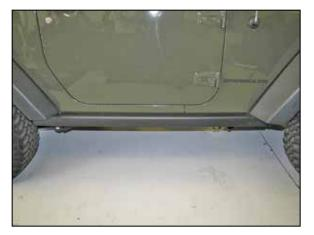
56. Reinstall the rock slider / running board if equipped.
