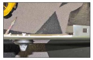
48. Using a cut-off wheel or similar tool, cut along the lines marked with the template and remove that section of the fender. Be sure to remove any remaining burrs with a file or deburring tool. **NOTE: After cutting it is recommended using paint to cover the exposed metal to prevent rusting of the fender.**
