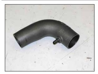
30. Install the provided NPT crank case vent fitting into the K&N<sup>®</sup> intake tube as shown. **NOTE: Plastic NPT fittings are easy to cross thread. Install the vent fitting "hand" tight, then turn it two complete turns with a wrench.**
