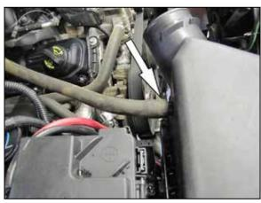
4. Disconnect the crank case vent hose from the upper air filter housing.
