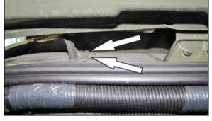
11. Lift up the cowl and then remove the two bolts that secure the fender to the inner cowl.
