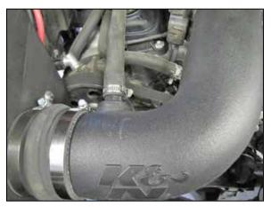
35. Install the provided crank case vent hose as shown and secure with the provided hose clamp.
