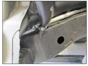
53. Install the duck bill fitting onto the port at the bottom of the corner tube and secure with the provided hose clamp.
