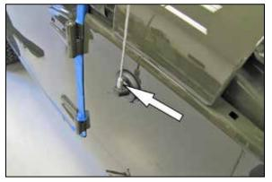
8. Remove the antenna mast.
