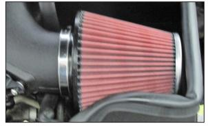
19. Install the K&N<sup>®</sup> air filter and secure with the provided hose clamp. **NOTE: Clock the filter for best fit.**
