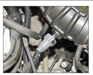
3. Disconnect the EVAP vent line by depressing the
