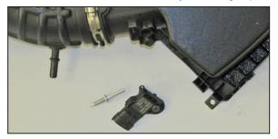
12. Remove the inlet temperature sensor from the upper air box.
