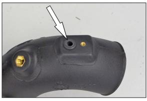
13. Install the provided grommet into the K&N<sup>®</sup> intake tube as shown.
