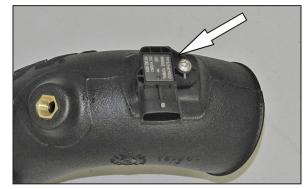
14. Remove the sealing O-Ring from the sensor and then install the sensor into the K&N<sup>®</sup> intake tube and secure with the provided hardware. **NOTE:** The sensor is a tight fit to prevent air leaks. Be careful so to not push the grommet through the hole when installing the sensor. Be sure to place the provided spacer between the sensor and tube before securing the sensor.
