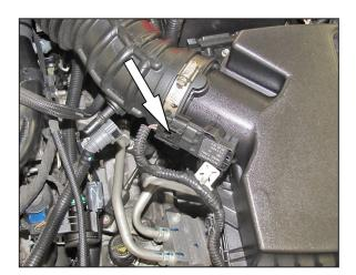
5. Disconnect the inlet air temperature sensor
