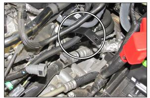
9. Be sure engine is completely cool before proceeding with this step. Remove the nut securing the thermostat housing (directly above the engine temperature sensor). Then install the provided tube mounting bracket and secure with the factory nut.
