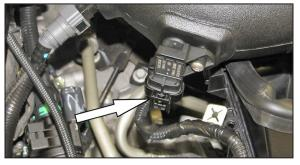
18. Reconnect the inlet air temperature sensor electrical connection.
