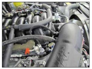
24. Connect the crank case vent hose and the fuel pressure hose to the fittings installed into the K&N® intake tube.
