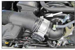
4. Loosen the hose clamp which secures the intake tube to the throttle body.
