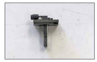
18. Install the mass air sensor assembly into the K&N® mass air sensor adapter as shown using the provided hardware.
