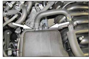
5. Disconnect the crank case vent hose and fuel pressure line from the intake resonator.
