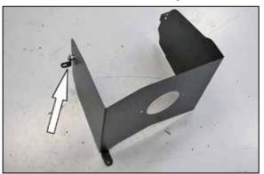
8. Install the heat shield mounting bracket (070066A) onto the heat shield using the provided spacer and hardware.
