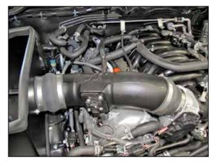
23. Install the K&N® intake tube into the hump hose at the heat shield and then into the step hose at the throttle body and secure with the provided hose clamp.
