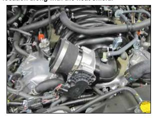
14. Install the coupler hose (08497) onto the throttle body and secure with the provided hose clamp.
