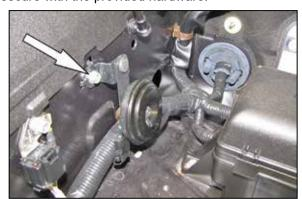
12. Remove the bolt which secures the horn to the inner fender.
