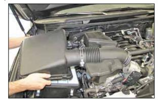
6. Release the four retaining clips securing the upper air box and then remove the upper air box and intake tube assembly from the vehicle.
