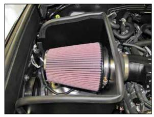
25. Install the K&N® air filter and secure with the provided hose clamp.
