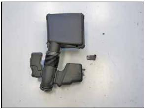
16. Remove the two screws securing the mass air sensor and then remove the mass air sensor from the upper air box housing.
