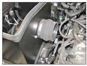
15. Install the hump coupler (08418) onto the filter adapter and secure with the provided hose clamp.
