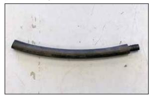
21. Install the hose mender into the provided crank case vent hose as shown.
