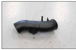
20. Install the provided NPT vent fittings into the K&N® intake tube as shown.
