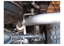
SLIDE PASSENGER SIDE TAILPIPE #E INTO MUFFLER 1-1/2" TO 2". USE CLAMP #I TO SECURE TAILPIPE TO MUFFLER. DO NOT TIGHTEN. INSERT HANGER INTO RUBBER GROMMET.
