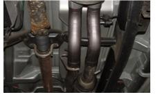
SLIDE PASSENGER SIDE HEADPIPE #A ONTO STOCK HEADPIPE. INSERT WELDED HANGER INTO RUBBER GROMMET. NEXT INSTALL DRIVERS SIDE HEADPIPE #B ONTO STOCK HEADPIPE, USE CLAMP #H TO SECURE BOTH HEADPIPES, DO NOT TIGHTEN.
