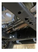
Install head pipe #A onto you're existing stock Pipe use your factory Band Clamp.
