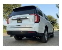
Finally, go back and tighten all clamps, nuts and bolts. Use stainless steel cleaner and a Scotch Brite pad weekly to prevent tip from discoloration. Inspect all fasteners after 25-50 miles of operation and retighten as necessary.
