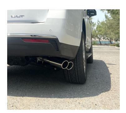
GIBSON EXHAUST systems are designed on a factory stock vehicle. Any aftermarket products installed could increase the sound levels of this Exhaust. Make sure there is a 1" clearance from ALL rubber brake lines, shock boots, fuel lines, tires, etc to prevent heat related damage or fire.
