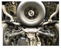
Re install spare tire and heat shield. Position all pipes and double check all connections prior to tightening clamps.
