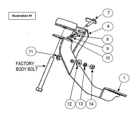
**Step-3** Remove the passenger side middle body mount bolt, (Photo 3).
