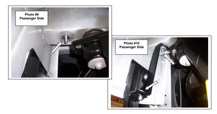
**Step-6** Position the frame bracket on top of the vehicle spring hanger so the slot hole in the bracket and hole in the spring hanger align. Attach the frame bracket to the spring hanger using (1)  $\frac{1}{2}$ " x 1" hex bolt, (1)  $\frac{1}{2}$ " flat washer and (1)  $\frac{1}{2}$ " flange nut. **Photo #11 & #12** Do not fully tighten at this time.
