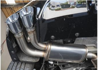
**Step 3.** Complete the installation by attaching the Muffler Assemblies to the Y-Pipe using the supplied 2.50" clamps. Engage the hangers into OE rubber insulators.
