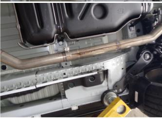
Step 2. Begin installation of the MagnaFlow system by attaching the Muffler Assembly to the outlet of the catalytic converter using the supplied 2.00" clamps. Next, attach the Extension Pipe and Y-Pipe Assemblies using the supplied 2.50" clamps and engaging the hanger into the rubber insulators. (Leave all clamp and fasteners loose for final adjustment of the complete system.)
