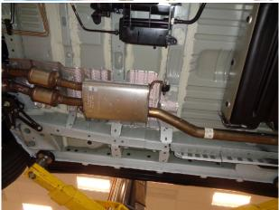
Step 1. To remove the OE exhaust it will need to be cut. Measuring back from the rear weld on the catalytic converters (in front of the muffler) cut the driver side 3.00" and the passenger 4.00" back from the welds as shown. Once cut, working front to rear disengage the hangers from the rubber insulators and remove the exhaust. Do not damage the rubber insulators as they will be used to install the new exhaust system.
