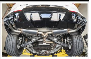
**Step 4.** Once a final position has been chosen for the new exhaust system, evenly tighten all clamps and fasteners, from front to rear, using the torque specifications on page one of the instructions. Inspect all fasteners after 25-50 miles of operation and re-tighten if necessary.
