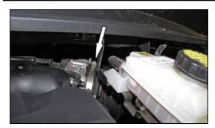
7. Loosen the hose clamp securing the factory intake tube to the throttle body and then remove it from the vehicle.
