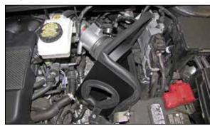
15. Install the heat shield assembly into the vehicle so the mounting studs insert into the factory air filter housing mounting studs and the intake tube inserts into the coupling hose. Secure the heat shield with the provided hardware then adjust the intake tube for best fit and secure with the provided hose clamps.
