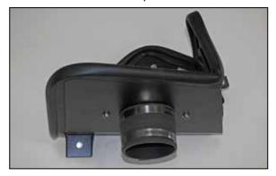
14. Install the provided coupler hose (08496) onto the filter adapter and secure with the provided hose clamp.
