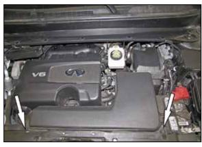
2. Remove the two bolts that secure the fresh air duct and then remove the fresh air duct from the vehicle.
