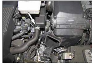
3. Release the spring clamp and then disconnect the negative battery cable.
