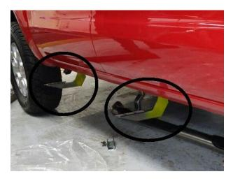
**Step-3** Attach the front bracket to the rocker panel using the install (2) M10 Hex nut (2) flat washer and (2) lock washer. **(Photo 3).**
