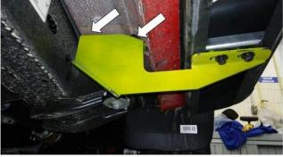
**Step-4** Install the RB10 or RB20 on the brackets installed using (6) M8-1.25 X 30mm Metric Hex Head Sems Bolts ( Photo 4).
