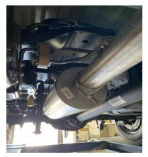
INSTALL MUFFLER # H ONTO HEADPIPE, USE CLAMP #D TO SECURE MUFFLER TO HEADPIPE. DO NOT TIGHTEN. USE A JACK STAND TO HOLD UP THE MUFFLER. OUTLETS SHOULD BE LEVEL.
