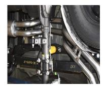
INSTALL PASS. SIDE TAILPIPE #B INTO MUFFLER. INSERT HANGER INTO RUBBER GROMMET, USE CLAMP #E TO SECURE PIPE TO MUFFLER. DO NOT TIGHTEN.
