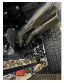
INSTALL DRIVERS SIDE TAILPIPE #C INTO THE MUFFLER, INSERT HANGERS INTO RUBBER GROMMETS, USE CLAMP #E TO SECURE PIPE TO MUFFLER. DO NOT TIGHTEN. THE TAB ON THIS PIPE SHOULD GO ON BOTTOM OF PASSENGER SIDE PIPE USE BOLT KIT #G TO SECURE TOGETHER.
