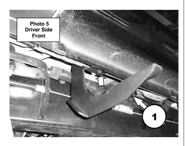
**Step-4** Locate the plastic plugs and holes in the rocker panel at the center and rear of the cab, and repeat steps1-3 to install the 3 additional brackets, (Photo 6 & 7). Leave the bolts loose for final adjustment.
