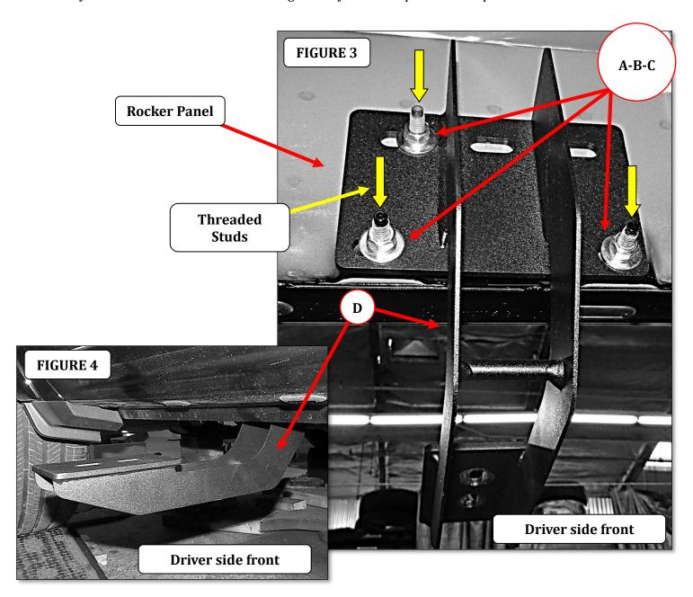
**Step-3** Locate the (3) threaded studs on the inner rocker panel at the center and rear of the cab and repeat step 2 to install two of the brackets using the supplied hardware. Note: The front mounting location is shown in Figure 3. The center and rear mounting locations are similar.
