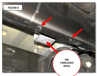
**Step-6** Attach one of the driver side Rear/Rear Center brackets to the pinch mold using (2) 1/4" x 1" hex head bolts, (4) 1/4" flat washers, (2) 1/4" lock washers and (2) 1/4" hex nuts, and to the underside of the body using (1) M8 x 25mm hex bolt, (1) 5/16" lock washer and (1) 5/16" flat washer, (FIGURE 9 & 10). Leave the nuts and bolts loose for final adjustment.
