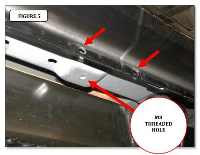
**Step-4** Attach one of the driver side Front/Front Center brackets to the pinch mold using (2) 1/4" x 1" hex head bolts, (4) 1/4" flat washers, (2) 1/4" lock washers and (2) 1/4" hex nuts, and to the underside of the body using (1) M8 x 25mm hex bolt, (1) 5/16" lock washer and (1) 5/16" flat washer, (FIGURE 6 & 7). Leave the nuts and bolts loose for final adjustment.
