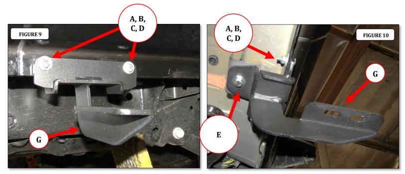
**Step-7** Locate the (2) holes in the body pinch mold and (1) M8 threaded hole in the underside of the body at the rear center of the vehicle, and repeat step 6 to install the remaining driver side bracket.
