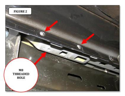
**Step-2** Attach one of the driver side Front/Front Center brackets to the pinch mold using (2) 1/4" x 1" hex head bolts, (4) 1/4" flat washers, (2) 1/4" lock washers and (2) 1/4" hex nuts, and to the underside of the body using (1) M8 SEMS BOLT (FIGURE 3 & 4). Leave the nuts and bolts loose for final adjustment.
