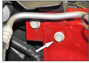
20. Remove the front fender mounting bolt shown. **NOTE: This bolt will be reused.**
