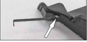
18. Install the heat shield mounting bracket (083103-1) onto the heat shield using the provided hardware.
