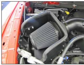
30. Install the K&N® air filter and secure with the provided hose clamp.
