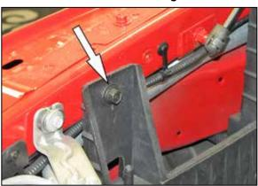
19. Remove the front air box mounting bracket bolt shown.
