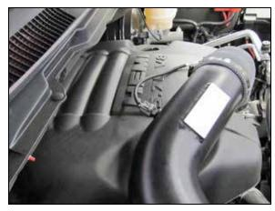
29. Choose the appropriate inlet air temperature sensor extension harness and then connect Install it too the inlet air temperature sensor and vehicle harness.
