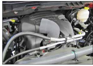
22. Install the provided silicone hose (08498) onto the throttle body and secure with the provided hose clamp
