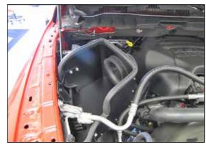
21. Install the heat shield into the vehicle and secure with the factory bolts from steps #19 and #20.
