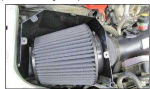
34. Feed the K&N® air filter top first into its location then rotate it back and install onto the filter adapter. Secure the air filter with the provided hose clamp.
