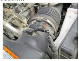
2. Release the red locking tab and then disconnect the mass air sensor electrical connection and unhook the wiring harness from the air box.
