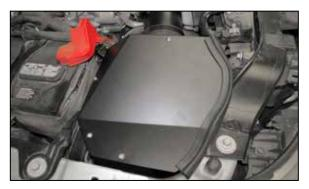
36. Install the heat shield lid onto the heat shield and secure with the provided hardware.
