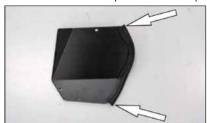
35. Install the provided edge trim onto the heat shield lid as shown.
