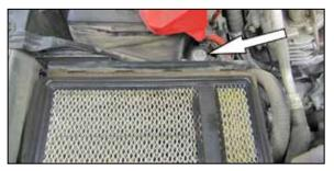
9. Remove the bolt securing the lower air box to the battery tray.
