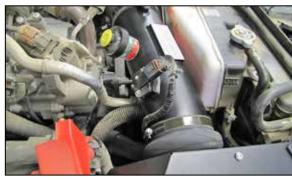
37. Reconnect the mass air sensor electrical connection.
