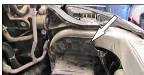
16. Remove the push pin securing the top of the fresh air intake duct.
