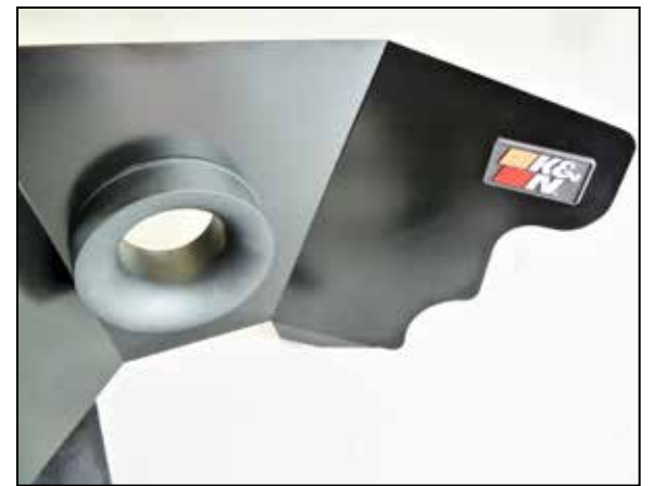
9. Install the provided couplers onto the turbo inlets and secure with the provided hose clamps.
