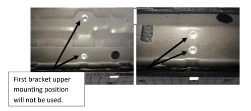
**Step 3:** Starting with the driver side, position step up to the body of the vehicle and align the brackets up with the factory mounting locations.
