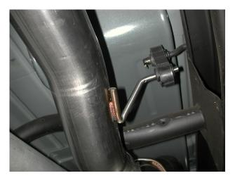
**Step 2.** Install corresponding Inlet Pipe Assembly. Loosely fasten it to the turbo charger outlet using the OEM clamp. Next, loosely attach the extension pipe assembly to the Inlet Pipe Assembly using the supplied clamp.
