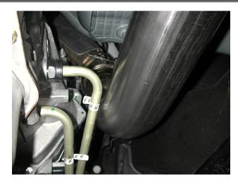
**Step 1.** Working front to rear loosen or remove all OEM band clamps and disengage all welded hangers from the rubber insulators. Be sure to retain all mounting hardware as it will be needed to install your new MAGNAFLOW system.
