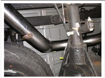
**Step 4.** Loosely install the Over Axle Pipe Assembly using the supplied Hanger Clamps
