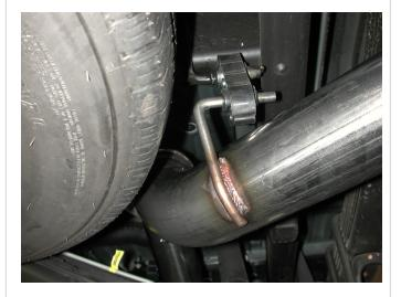
**Step 5.** Install the Tail Pipe Assembly in the same way. The Outlet may be trimmed as desired.
