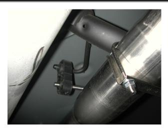
**Step 3.** As you assemble the Extension Pipes loosely locate the Hanger Clamp Assemblies as needed.
