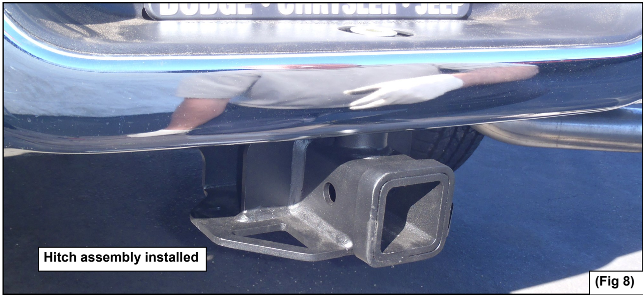
Re-install bumper cap (Note: If bumper cap does not fit then use provided bumper cap instead (Item 8))
