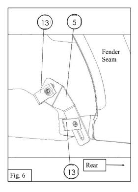
9. Next, install the Inner Fender (1) and line it up with the mounting brackets and U-Clip on the body of the vehicle. *Note:* It is necessary to bend the rear inner fender in order to place it inside of the wheel well. Removing the tire may make installation easier.
