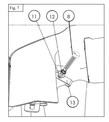
10. Secure with the provided M6 Hardware. *Note:* Make sure that the top of the Rear Inner Fender is pressed up against the back of the wheel well. Use Short M6 Button Head Screws (9) to attach rear inner fender to brackets. See Figures 8 & 9. See Figures 10 & 11 for M6 hardware model.
