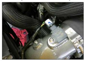
21. Reconnect the pressure sensor electrical connection.
