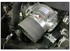
15. Install the provided step hose onto the throttle body and secure with the provided clamp.
