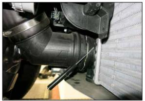
8. Using a small screwdriver or similar tool, release the locking clip that secures the factory charge tube to the intercooler and then disconnect the tube
