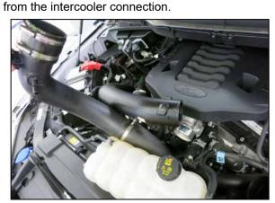
9. Remove the factory charge tube from the vehicle.
