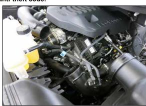
2. Loosen the three hose clamps that secure the factory intake tube to the turbo inlet tubes and air filter housing and then remove the intake tube from the vehicle.
