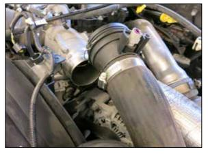
6. Separate the charge tube from the throttle body.
