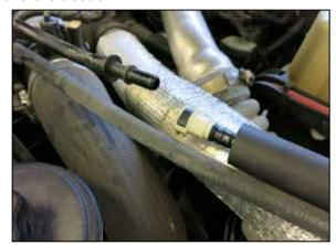
2. Disconnect the vent line at the quick connect fitting.
