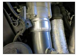
13. Connect the quick connector to the throttle body, push the coupler firmly until there is an audible "click" is heard. Pull back on the coupler to be sure the locking ring is engaged.
