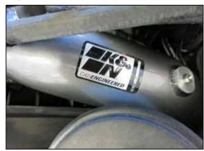
17. Install the provided 1/8" npt plug and K&N decal. Be sure to apply thread sealer to the npt threads.
