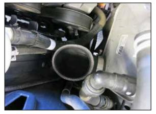
9. Install the provided elbow coupler onto the intercooler with the provided clamp but do not tighten completely.
