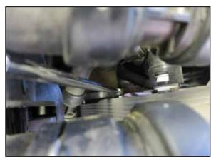
5. Using a 7mm socket, loosen the factory hose clamp that secures the charge tube to the inter cooler.
