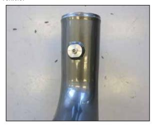
11. Install the provided 1/8npt pipe plug into the accessory port. Be sure to apply pipe thread sealant.
