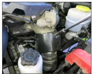
4. Remove the bolt that secures the throttle body cover and then remove the cover from the vehicle.
