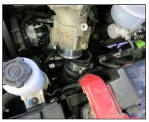
8. Disconnect the factory charge tube from the throttle body.
