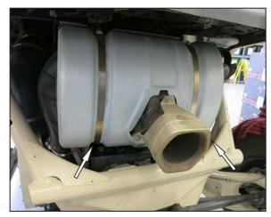
21. Reinstall the muffler using the factory hardware and springs. Reinstall the plastic muffler cover.
