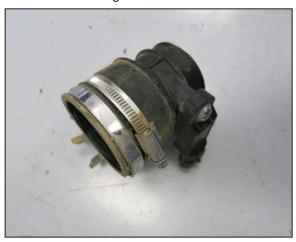
10. Remove the pressure sensor housing from the throttle body.
