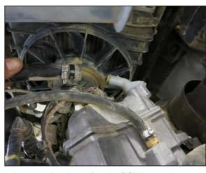
13. Loosen the clamp for the CCV hose, disconnect the hose from the engine and set aside.
