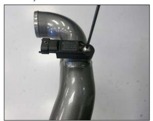
11. Remove the pressure sensor from the factory housing and install it into the K&N charge tube using the provided hardware.
