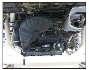
6. Disconnect the throttle body and pressure sensor electrical connection.
