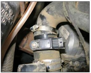
7. Loosen the hose clamps at the throttle body and the pressure sensor housing.
