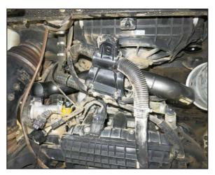
14. Install the K&N charge tube by routing it behind the factory plastic charge tube holder.
