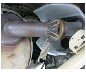
4. Remove the spring that secure the muffler to the flex joint and then remove the muffler from the vehicle.
