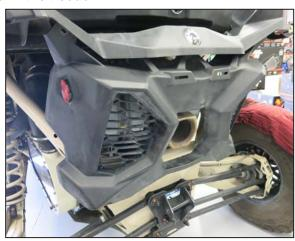
2. Remove the rear plastic exhaust cover and set aside.
