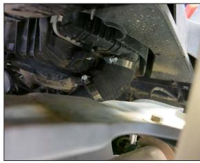
16. Insert the charge tube into the elbow coupler at the inter cooler.
