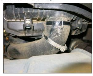
8. Loosen the hose clamp that secures the charge tube to the intercooler. Disconnect the charge tube plastic mounting bracket.
