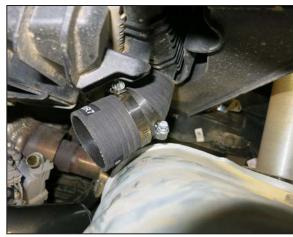
15. Install the elbow coupler onto the inter cooler with the provided hose clamps.
