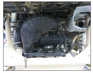
5. Loosen the clamp that secures the CVT breather hose and then remove the hose from the vehicle.
