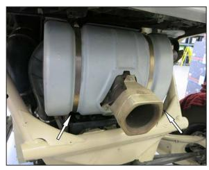
3. Remove the bolts that secure the lower muffler bracket.
