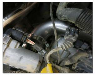
20. Reconnect the throttle body and pressure sensor electrical connections.
