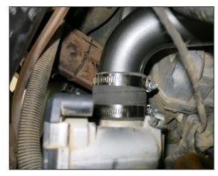
17. Insert the charge tube into the coupler at the throttle body, adjust the charge tube and couplers for best fit and then secure the hose clamps.
