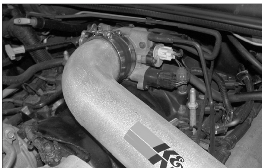
20. Slide the K&N® intake tube into the silicone hose on the throttle body and secure the bracket to the alternator using the stock bolt removed in step 18.
