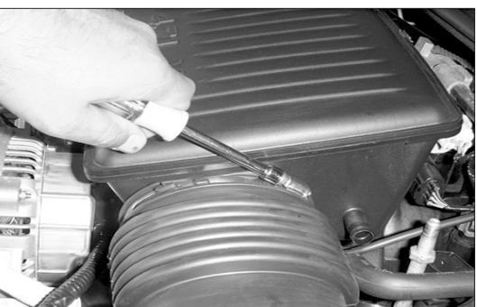
3. Loosen the hose clamp on the intake hose at the intake tube.
