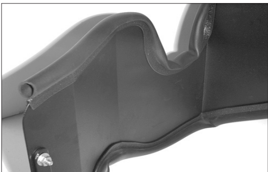
14. Install the trim seal onto the heat shield as shown. NOTE: Some trimming of the edge trim will be necessary.
