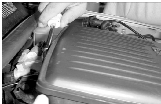
6. Loosen the hose clamp on the intake tube at the throttle body.
