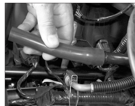
25. On 2003 models slide the silicone hose from step 24 onto the crank case vent hard line as shown.
