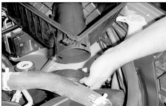
11. Detach the air inlet duct from the air box base and remove the air box base.
