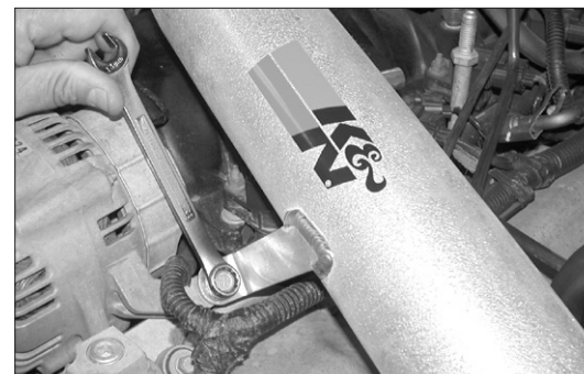
21. Adjust everything for best fit and clearance then tighten the alternator bolt as shown.
