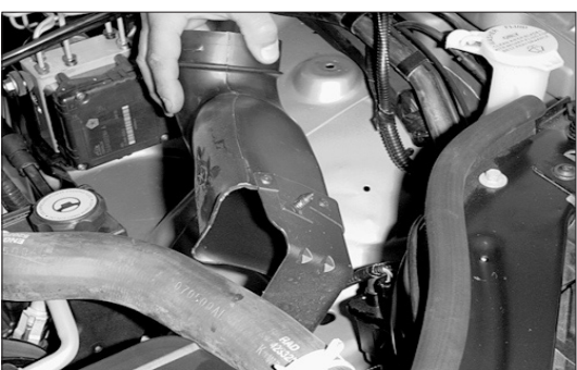
12. Release the clip that retains the air inlet duct to the radiator core support and remove the air inlet duct.
