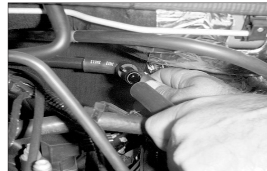
22. Attach the vent hose provided to the "T" fitting.
