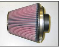
24. Install the provided filter adapter into the K&N<sup>®</sup> air filter and secure with the provided hose clamp.
