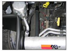
23. Install the provided silicone hose onto the fitting on the K&N<sup>®</sup> intake tube and then attach the open end onto the hose to the factory crankcase tube.
