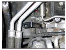
15. Install the tube mounting bracket onto the A/C compressor using the bolt removed in step #14 as shown.
