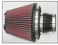
25. Install the silicone hose (08724) onto the air filter adapter as shown and secure with the provided hose clamp.
