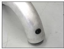
17. Install the provided grommet into the  $K\&N^{\otimes}$  intake tube as shown.
