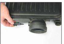
18. Twist the air temperature sensor counter clockwise and remove it from the stock intake plenum.
