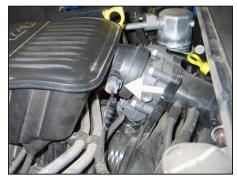
4. Depress the locking tab on the air temperature sensor electrical connection and disconnect the electrical connection.
