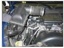
3. Disconnect the stock intake tube from the intake plenum. Then lift to remove to remove the airbox assembly from the vehicle as shown.
