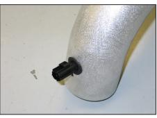
20. Install the air temperature sensor into the grommet installed into the K&N $^{\circ}$  intake tube in step #17.
