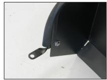
9. Install the twist bracket (070702) onto the heat shield with the provided hardware as shown.
