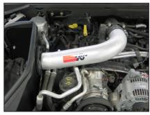
21. Install the K&N<sup>®</sup> intake tube into the into the silicone hose on the throttle body and position so the tube aligns with the mounting bracket. Secure the tube with the provided hose clamp and hardware.
