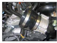
23. Install the provided silicone hose (08050) onto the throttle body as shown, secure with the provided hose clamp.
