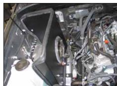
19. Set the heat shield into position on the inner fender and then secure with the factory bolt removed in step #18 and the provided hardware.
