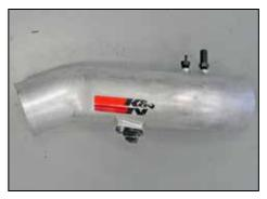
22. Install the provided NPT fittings into the K&N® intake tube as shown.
