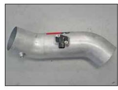
21. Install the mass air sensor into the  $K\&N^{\otimes}$  intake tube and secure with the provided hardware.
