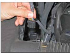
5. Disconnect the mass air sensor electrical connection and unhook the wiring harness from the upper airbox.
