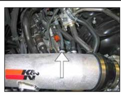
28. Reconnect the fuel pressure regulator vent line to the NPT fitting as shown.
