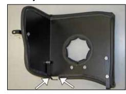
17. Install the provided longer edge trim onto the heat shield as shown.
