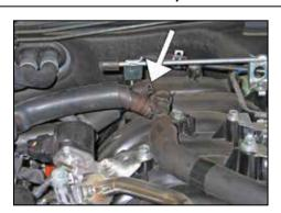
4. Disconnect the crankcase vent hose from the TEE fitting on top of the intake manifold plenum.
