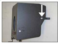
14. Install the provided heat shield mounting bracket (070742A) onto the heat shield using the provided hardware and spacer as shown.
