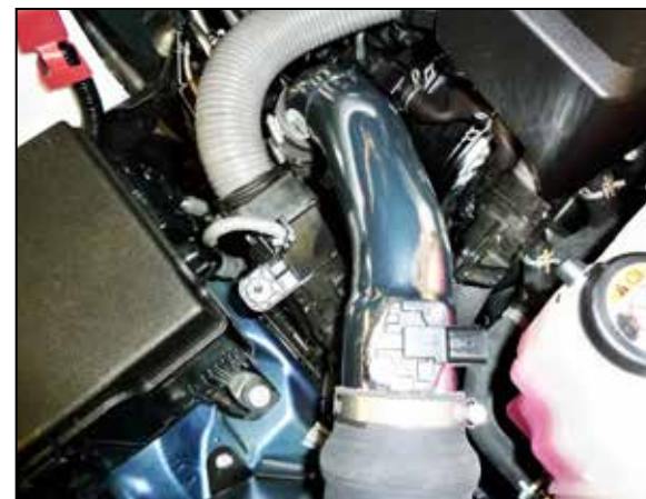
20. Install the passenger side intake tube into the couplers, adjust the tube for best fit and then secure with the provided hose clamps.
