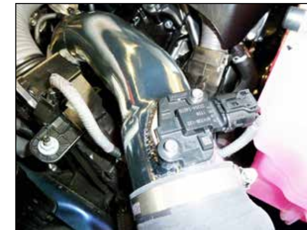
23. Reconnect the mass air sensor electrical connections.
