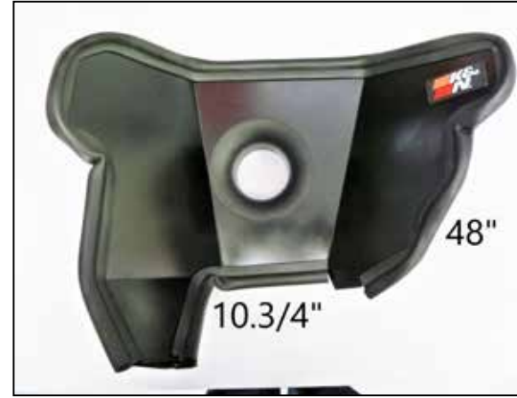
11. Cut the 61" L edge trim to lengths of 10.75" and 48", install the edge trim onto the driver side heat shield as shown.
