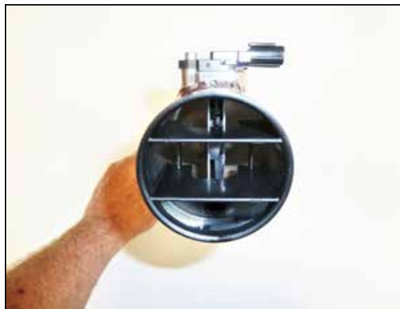
18. Install the air straighteners into the K&N intake tubes so that the blades are aligned as shown in relation to the mass air sensor.
