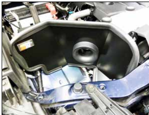
14. Install the passenger side heat shield assembly and secure with the provided hardware.
