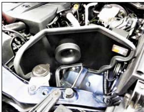
13. Install the driver side heat shield assembly and secure with the provided hardware.
