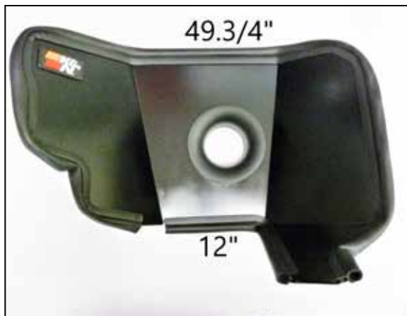
12. Cut the 66\"L edge trim to lengths of 12\" and 49.75\", install the edge trim onto the driver side heat shield as shown.
