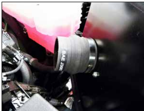
15. Install the provided hump couplers onto the filter adapters and secure with the provided hose clamp.
