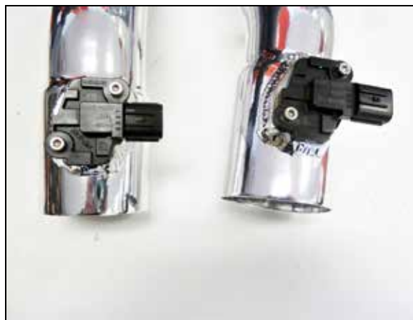
16. Remove the mass air sensors from the factory housings and install them into the K&N intake tubes using the provided hardware.
