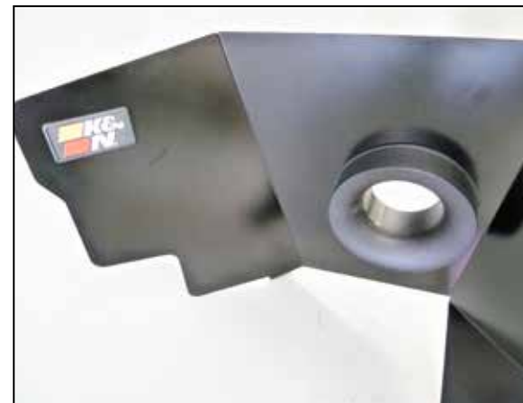
10. Install the filter adapters and K&N badges onto the heat shields using the provided hardware.
