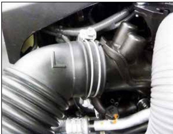
4. Loosen the hose clamps that secure the factory upper intake tubes and then remove the upper housings and intake tubes.
