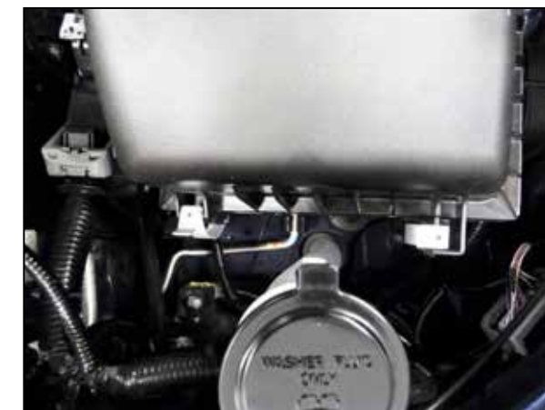
3. Release the retaining clips that secure the upper air filter housings.
