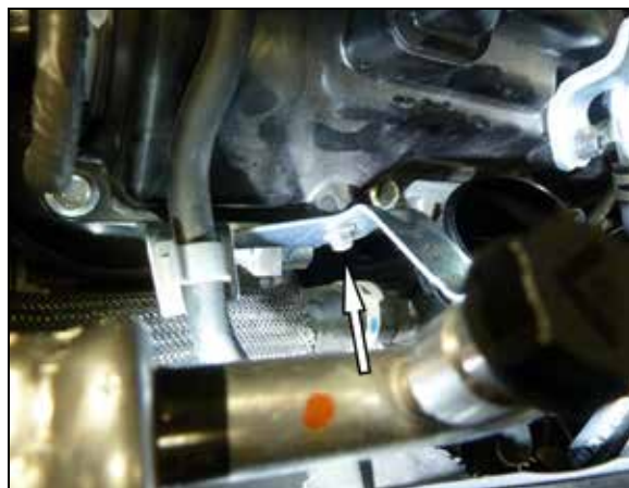
7. Remove the bolt that secures the driver side intake tube mounting bracket and then remove the bracket from the vehicle.
