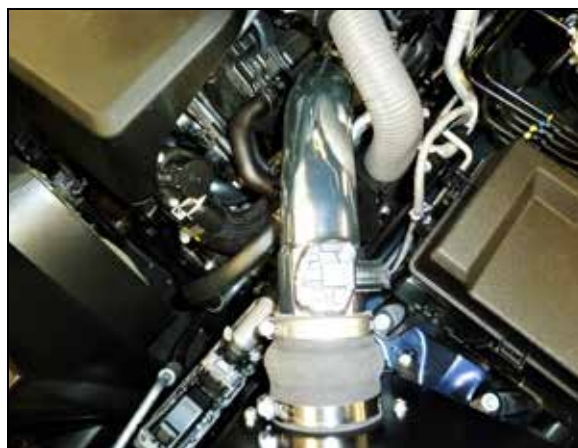
19. Install the driver side intake tube into the couplers, adjust the tube for best fit and then secure with the provided hose clamps.
