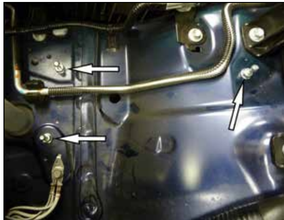
7. Remove the bolt that secures the driver side intake tube mounting bracket and then remove the bracket from the vehicle.
