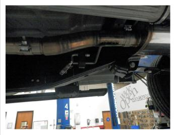
**Step 2.** Install the new system by attaching the Inlet Pipe Assembly to the resonator outlet pipe using the existing clamp. Locate the welded hanger to the rubber insulator. Leave all clamps and fasteners loose for final adjustment of the complete system once installed.
