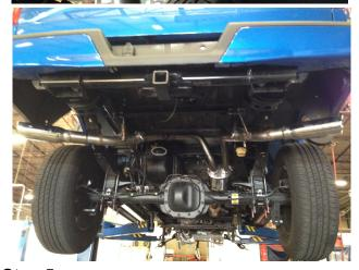
**Step 5.** To allow for the installation of a dual outlet system on a single outlet vehicle you will have to mount the supplied Hanger Brackets to existing holes in the factory frame rails using the supplied fasteners (8mm bolt and panel nut) as shown in the photos. Once completed you can now slide the Tailpipe assemblies onto the Over Axle pipes and fasten with the supplied 2.50" clamps and mount the hangers to the installed hanger brackets using the supplied rubbber insulators.
