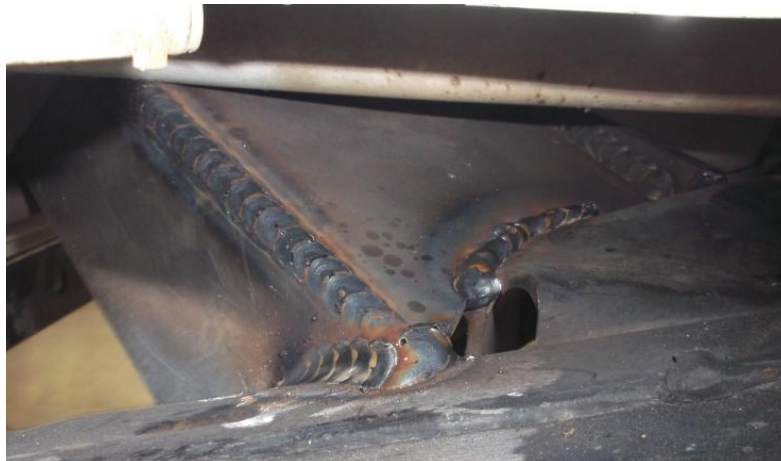
Figure 16. Upper Shock Mount Fully Welded
