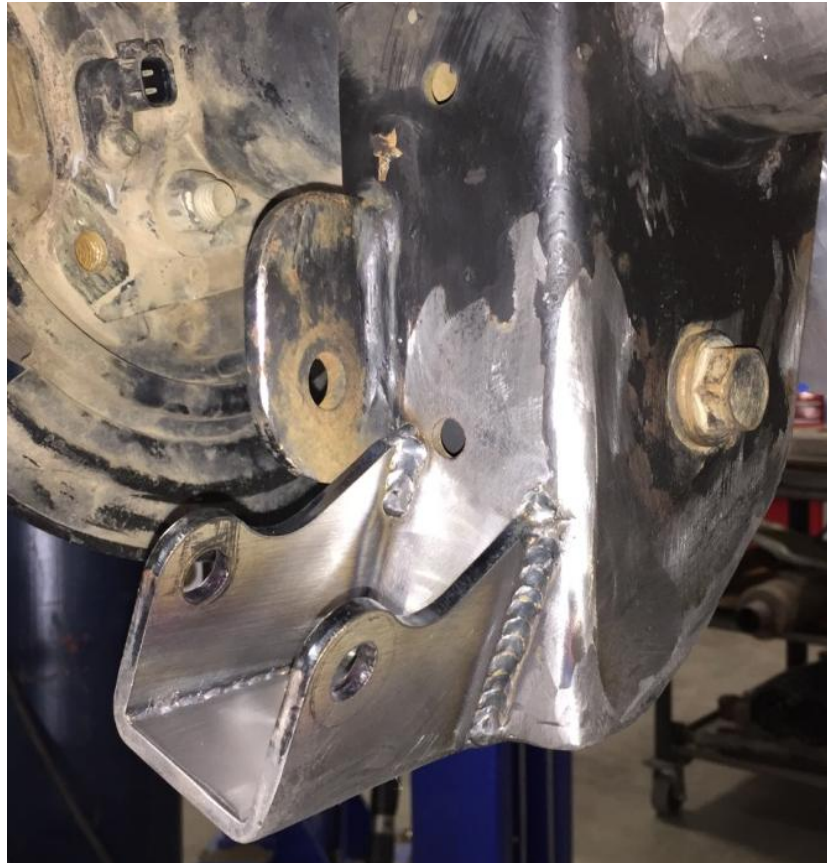
Figure 13. Lower Shock Mount Fully Welded
