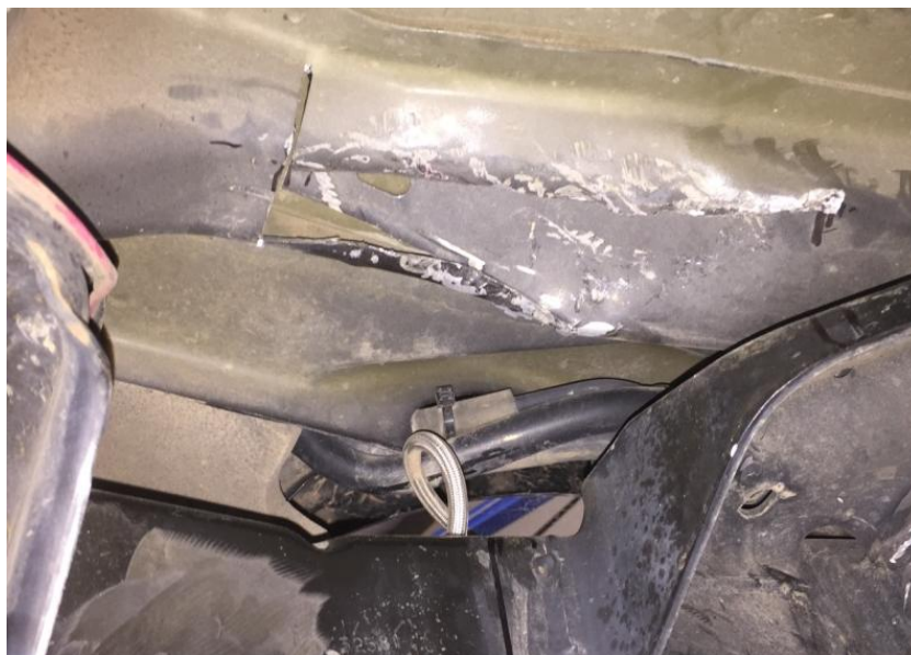
Figure 9. Trimmed Body to Allow for Upper Shock Mount Fitment
