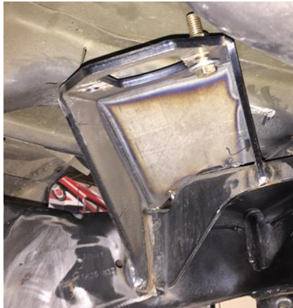
Figure 10. Shock Mount in Correct Position
