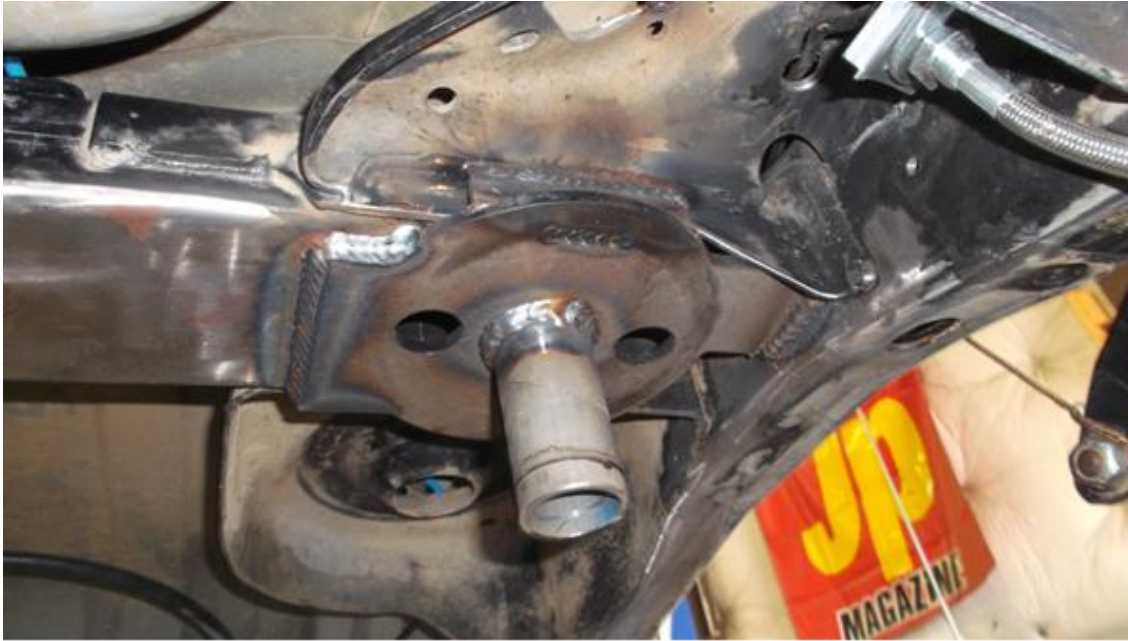
Figure 6. Rear View of Fully Welded Coil Mount
