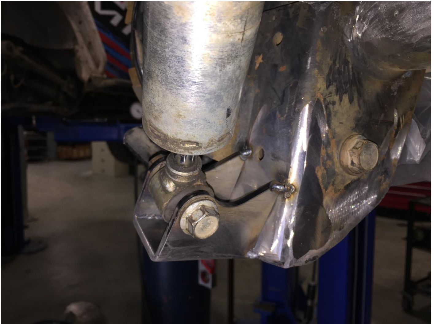
Figure 12. Lower Shock Mount tack welded to lower control arm mount.
