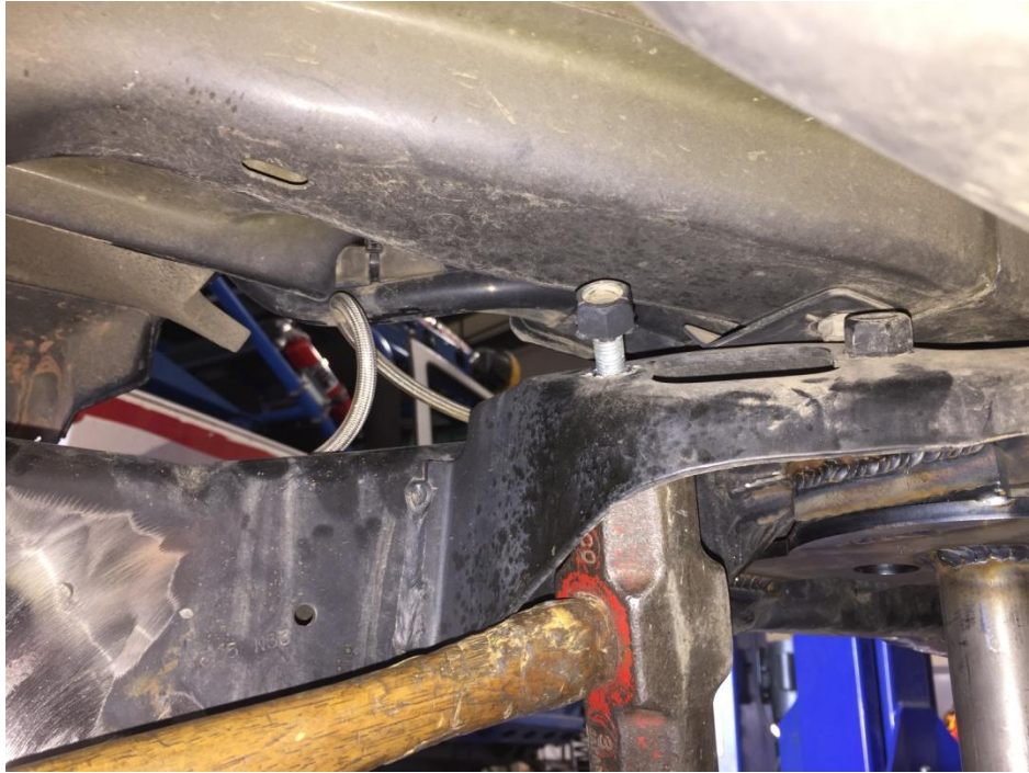
Figure 8. Removing the Stock Inner Shock Mount Nut
