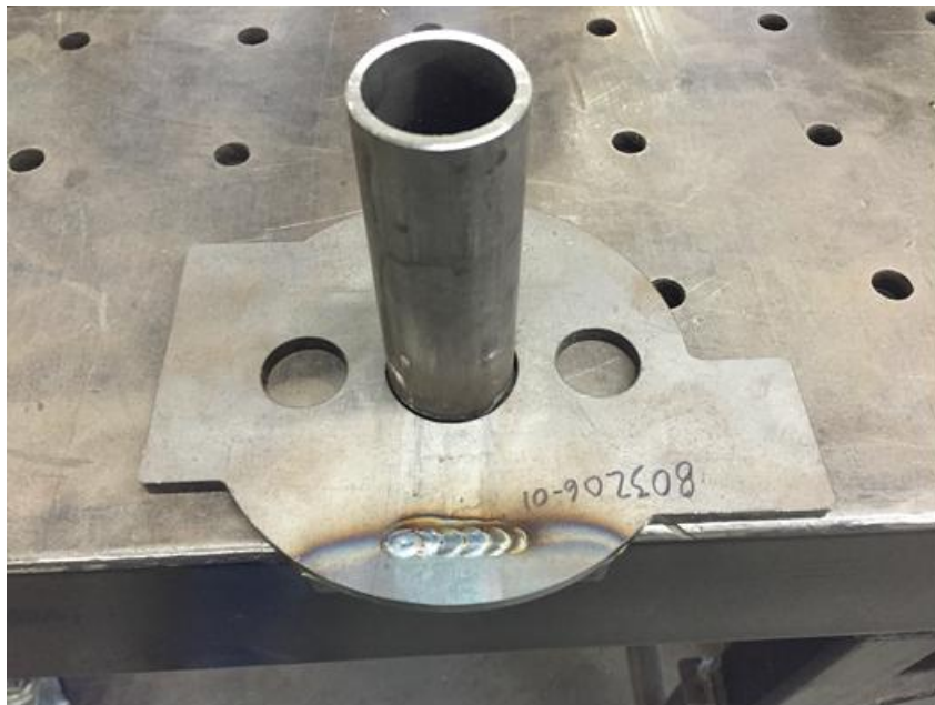
Figure 5. Locating Tube Positioned in Coil Mount
