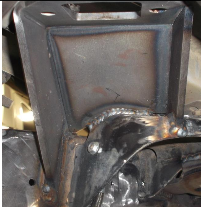
Figure 15. Upper Shock Mount Fully Welded
