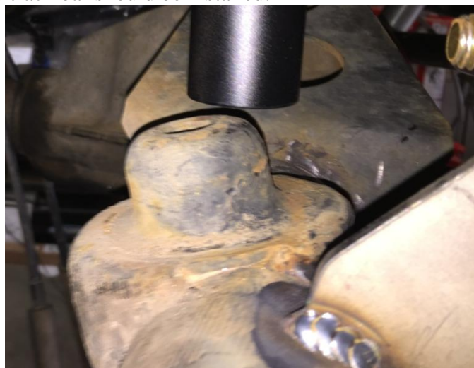
Figure 11. Coil Locating Tube in Relation to Axle Coil Mount at Bump
