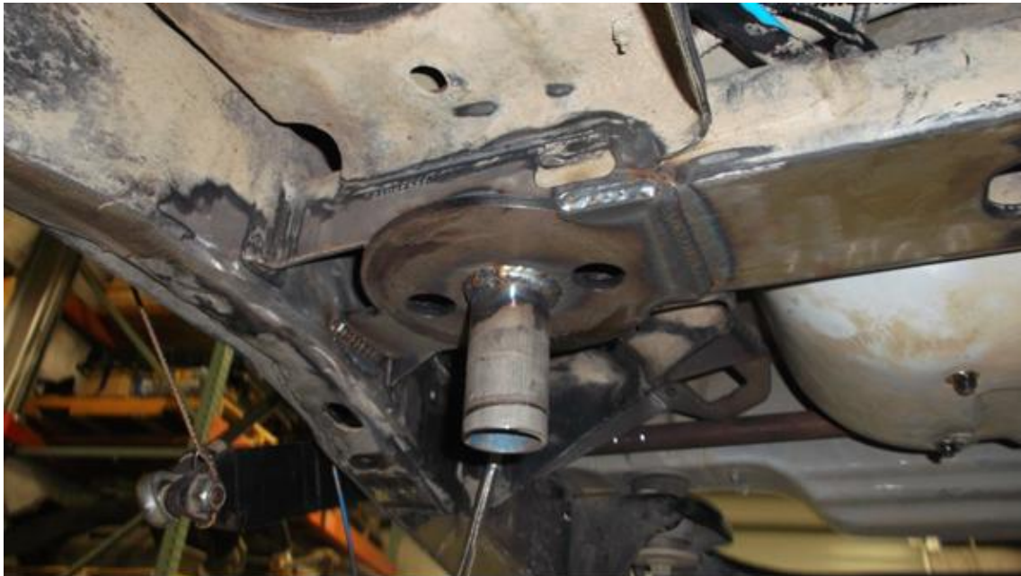
Figure 7. Front View of Fully Welded Coil Mount
