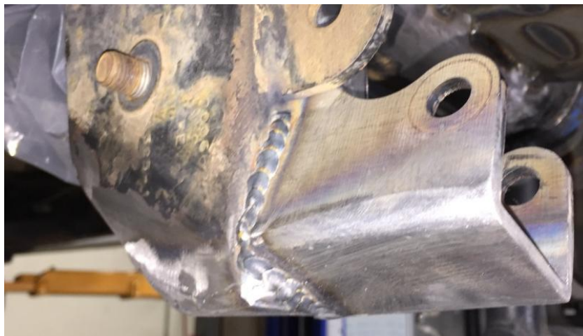
Figure 14. Lower Shock Mount Fully Welded
