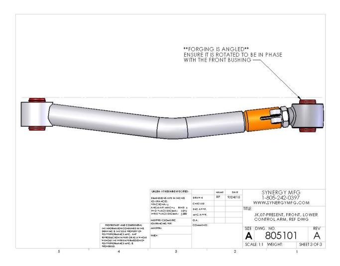
5. Install the new control arms with the adjuster at the frame end. The arms are bent in for tire clearance, and up for ground clearance. Be sure to install them correctly. Reuse the factory mounting bolts.
