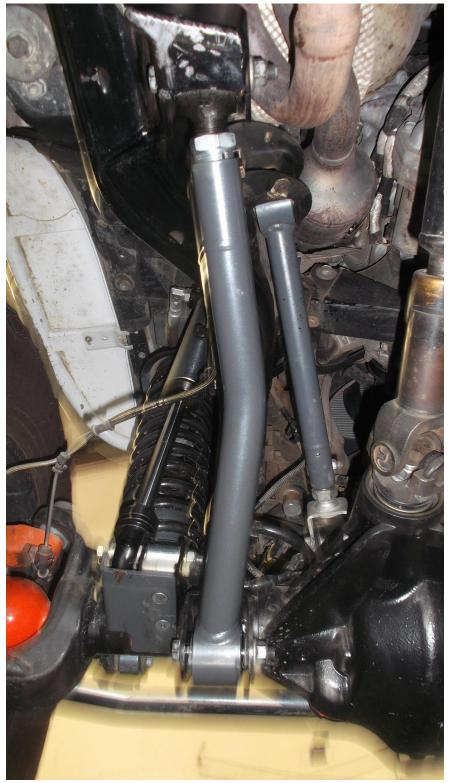
6. Tighten the factory control arm bolts to 125 ft-lbs. Once final length adjustments are made, ensure the vehicle is at ride height and tighten the pinch bolt to 80 ft-lbs. Put a wrench on the adjuster sleeve at this time and try to move the adjuster. Make sure pinch bolt has adequately clamped onto the flex joint shank so that the adjuster is not movable. If movable, increase torque on pinch bolt but do not exceed 90 ft-lbs.
