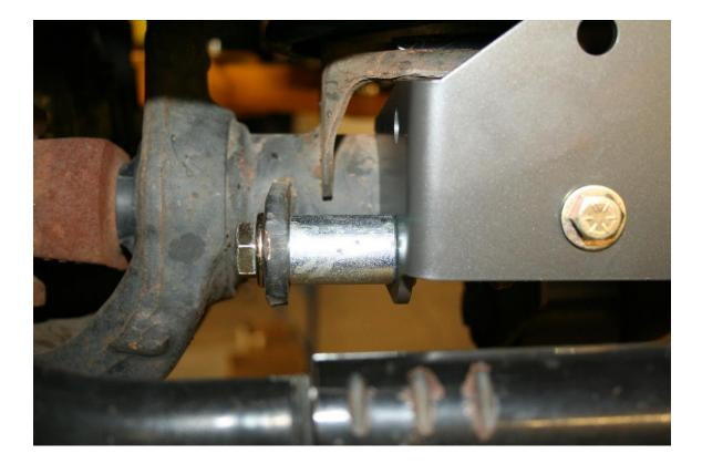
8. Install the driver side anti-sway bar relocation bracket using a 1.5"spacer and ½" x 3" bolt and top-lock nut; use a washer under the bolt-head and nut.
