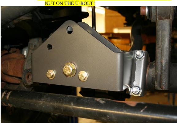
BE SURE TO USE THE 3/8-16 COARSE THREAD NYLOCK NUT ON THE U-BOLT!
