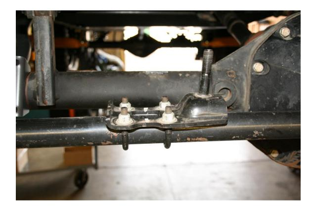
12. Install the steering stabilizer to the tie rod bracket. Attach the shaft end of the steering stabilizer to the track bar relocation bracket using the factory nut and bolt and a <sup>1</sup>/<sub>2</sub> washer between the bushing and the track bar relocation bracket.
