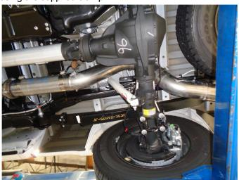
**Step 4.** Loosely install the Over Axle Pipe Assembly using the supplied clamp. Locate the welded hangers to the rubber insulators.
