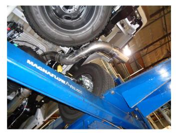
**Step 5.** Loosely install the Tail Pipe Assembly using the supplied clamp. Engage the welded hanger to the rubber insulator.
