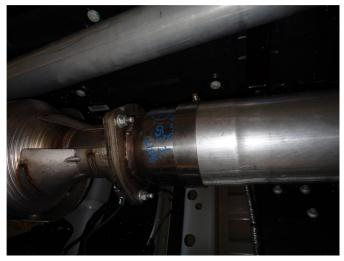
**Step 3.** Begin installation by loosely attaching the Inlet Pipe Assembly to the OEM flange outlet using the OEM hardware. Loosely attach the Extension Pipe, if needed, using the supplied clamp.
