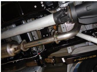
**Step 1.** To remove the OEM exhaust remove the O2 sensor from the over axle pipe. Unbolt the extension pipe assembly from from the DPF outlet flange and the OE over axle pipe. Working front to rear disengage all welded hangers from the rubber insulators. Be sure to retain all mounting hardware as it will be needed to install your new MAGNAFLOW system.
