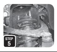
A coil/strut compressor will need to be used to contain and colapse the coil safely.
